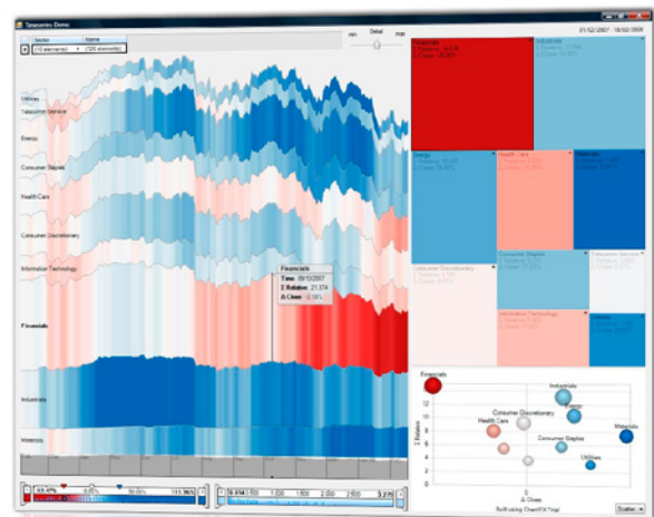
This multiple visualization view shows the performance of a fund across time. The Treemap and Scatter Plot highlight overall sector performance and correlations. The Stack Graph shows the performance every day across the year. From this screen, the user can drill into a sector to see the constituent stocks and their relative performance across time.
